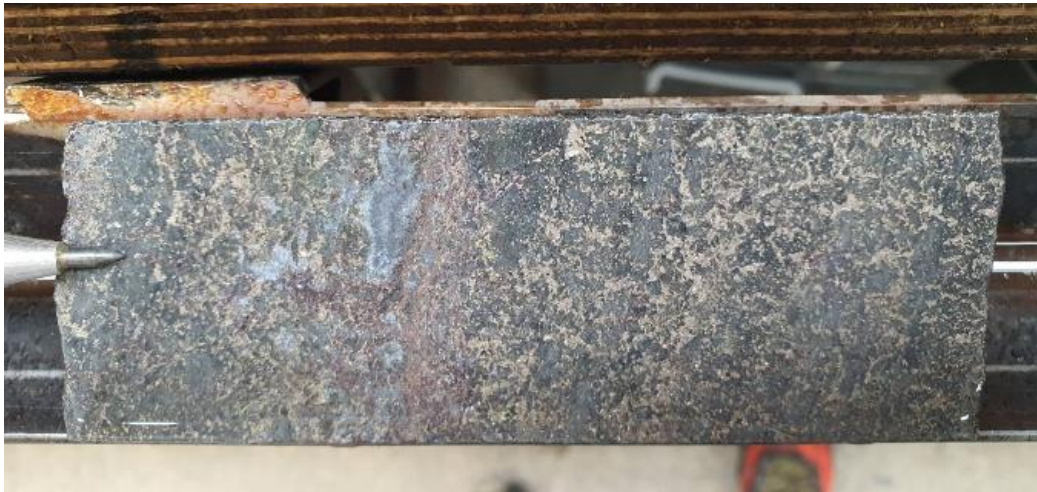
Figure 9. Close-up photo of the E-lode sulphide mineralisation from drill hole HAM0001 at 191.6 m, showing pyrrhotite and sphalerite with minor chalcopyrite with strong actinolite alteration and silicification.
