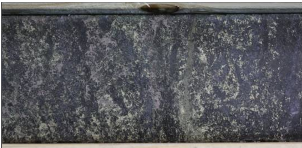
Figure 3: Examples of the E-lode sulphide mineralisation intersected in drill hole HAM0008.
