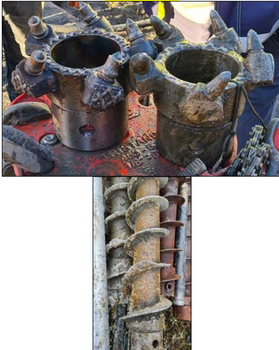
Figure 1: New auger bit (left), used auger bit (centre), damaged auger flyte (right)
