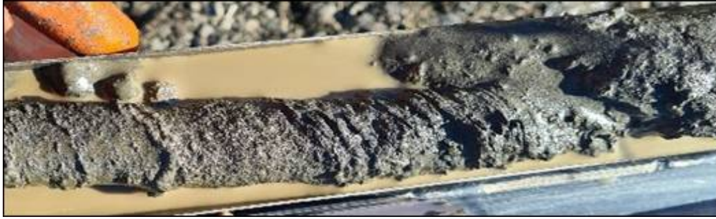
Figure 3: Diamond coring samples showing preferential washing of sand, reduced sample quality.
