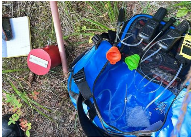
Figure 4: Helium Detector being prepared for casing vent test
