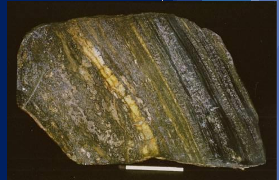
Finely laminated Zn-Pb mineralisation from the Kangerluarsup Glacier Showings, Kangerluarsuk
